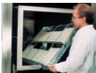
Figure 1 Loading a 1 \text{ m}^3 test chamber with adhesive on glass plates
