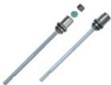
Figure 2 Left: Exploded view of transport adapter for automated liner exchange with liner, adapter, 3 x 5mm septum and septum screw; a hole for carrier gas entry can be seen between the o-rings of the transport adapter. Right: Assembled transport adapter with liner
