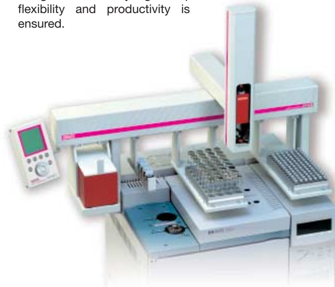
High Productivity autosampler for liquid injection and Large Volume Injection: MPS 2
