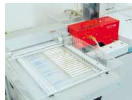
Figure 3 GERSTEL TDS system with autosampler mounted on 6890 GC with 5973 MSD
